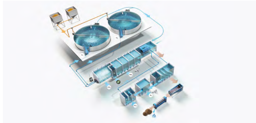
Figure 28 - The zero-water exchange concept (ZWC) is placed in between the RAS and the final wastewater treatment.
